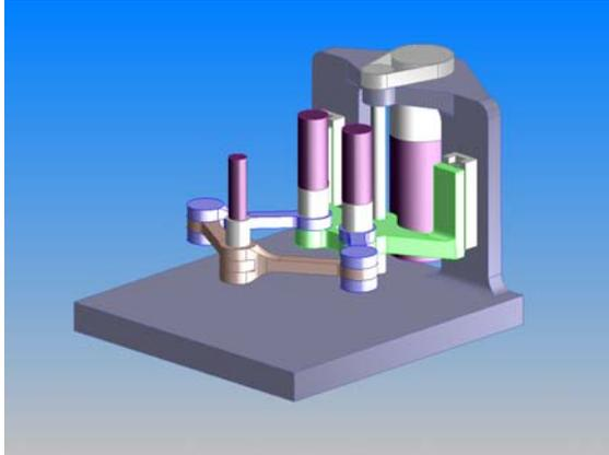
Fig 3: Concept for parallel SCARA structure
