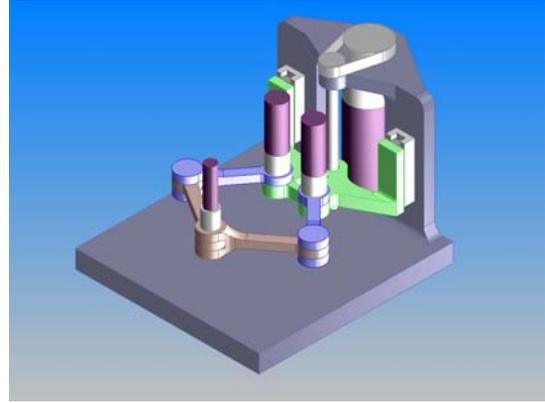
Fig. 11: Design alternative – ballscrew drive for Z-axis
