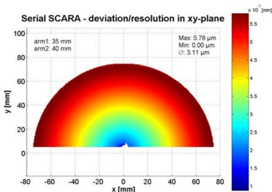
Fig 4: Resolution for serial SCARA (x-direction)
