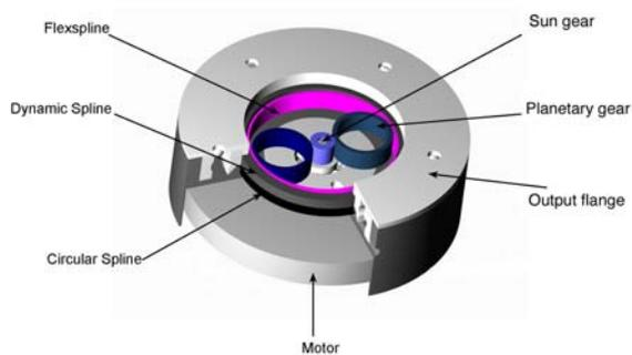
Fig. 7: Micro Harmonic Drive<sup>®</sup> gear components
