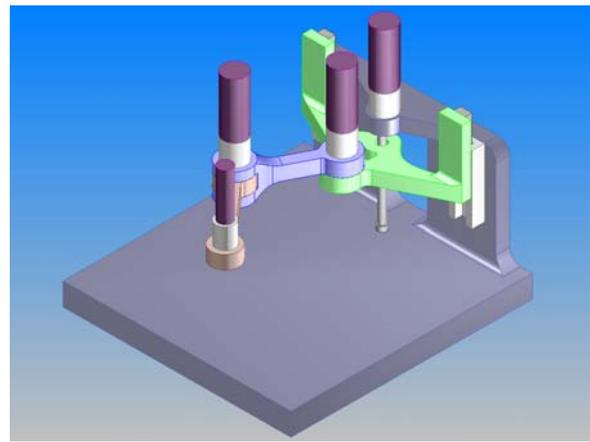
Fig 2: Concept for serial SCARA structure
