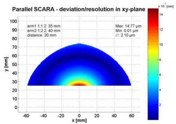
Fig 5: Resolution for parallel SCARA (x-direction)
