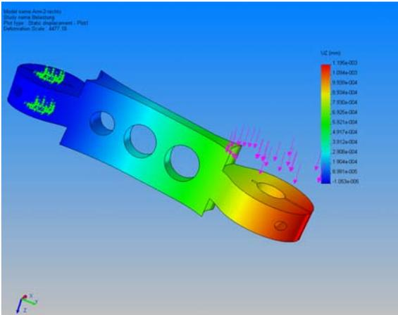
Fig. 9: FEM Lower arm displacement for load of 0.5N
