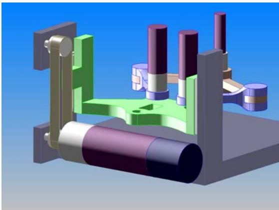
Fig. 10: Design alternative – Belt drive for Z-axis
